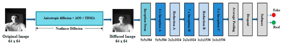
Figure 2. End-to-end architecture using the Inception v4 network.
