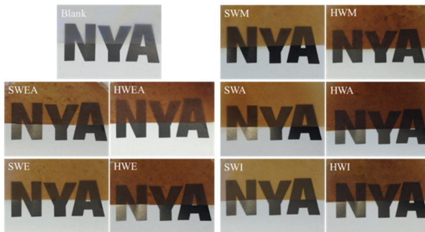
Figure 3. Digital photos of CNF-starch film and composite films containing different lignin fractions of spruce and eucalyptus lignin.
