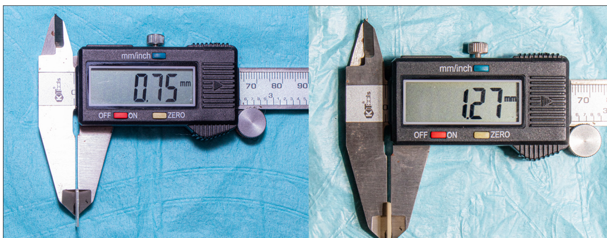
Figure 1. Measuring of thickness (0.07 and 1.00 mm) ceramic laminate veneer by using a digital micrometer.
