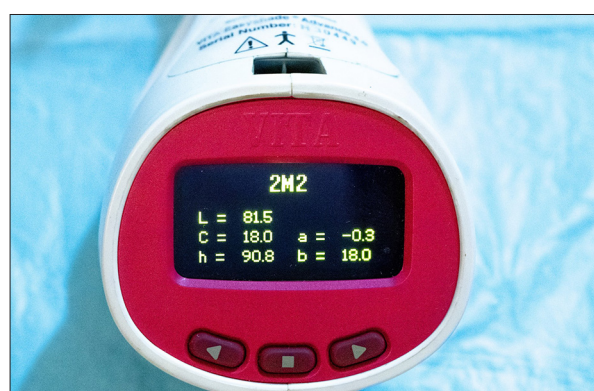
Figure 2. Reading of color parameters from VITA Easy-Shade spectrophotometer.
