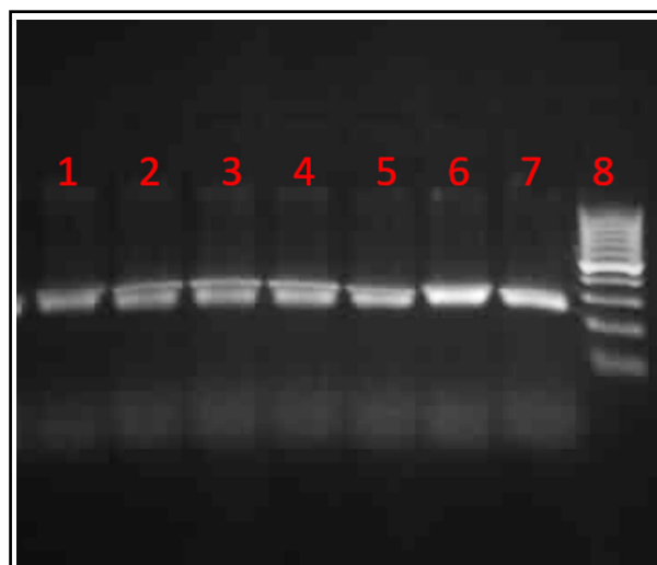
Fig.2: Genotyping of exon 7 polymorphism (rs1801725) in CASR gene. This gel represents the PCR products after digesting with Hin II enzyme. Lanes (1-5) showed heterozygous genotypes with three bands of sizes (28, 241, and 269 bp). Lane 6 showed homozygous genotype with one band of size (269 bp). Lane 8 represents the DNA ladder (100 bp).
