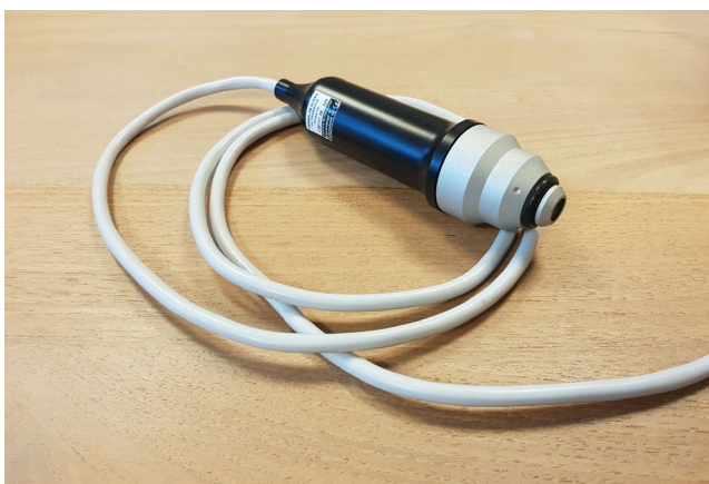
FIGURE 1 20-MHz echoprobe to measure skin thickness, DermaLab Combo® [Colour figure can be viewed at wileyonlinelibrary.com ]
