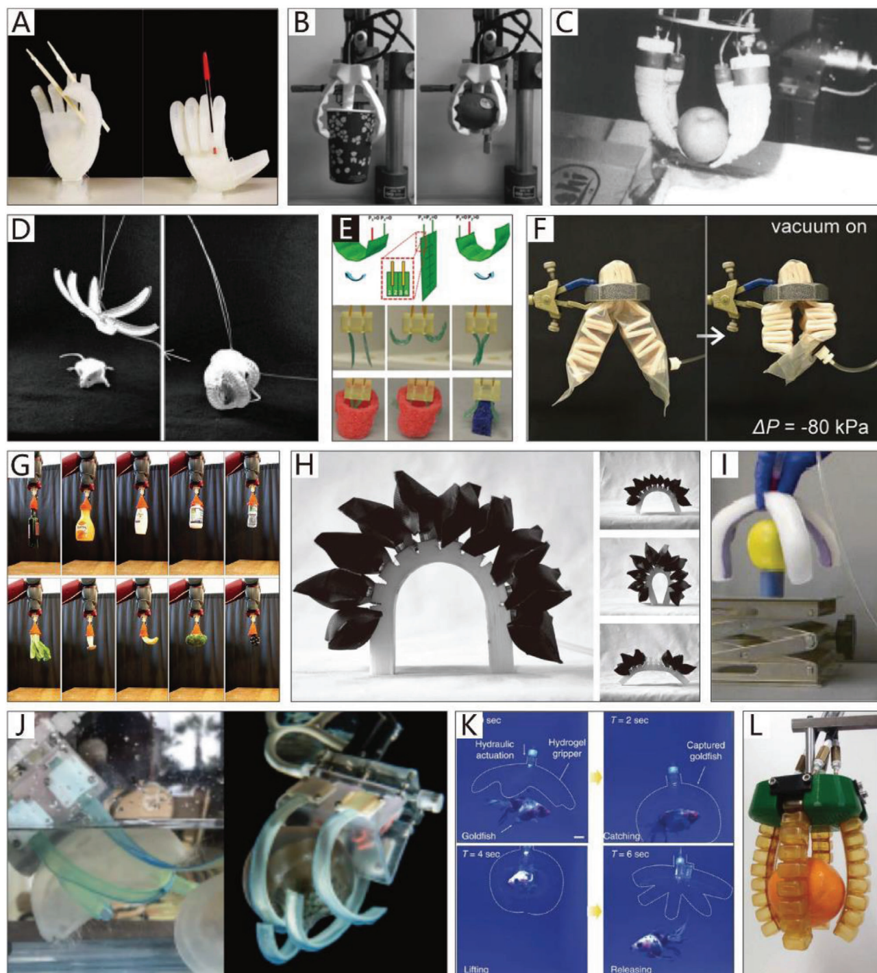
Figure 5. CBGs based on SPAs. A) A dexterous robotic hand driven by a PneuFlex actuator. Reproduced with permission. [140] Copyright 2016, SAGE Publications. B) A bio-inspired 3D printable soft vacuum gripper. Reproduced with permission. [141] Copyright 2018, Mary Ann Liebert, Inc. C) A flexible pressure-driven gripper. Reproduced with permission. [54] Copyright 1990, Cambridge University Press. D) A starfish-like gripper. Reproduced with permission. [108] Copyright 2011, John Wiley and Sons. E) A pressure-driven gripper with bilaterally curved fingers. Reproduced with permission. [81] Copyright 2017, Mary Ann Liebert, Inc. F) A gripper with asymmetrical beam structure. Reproduced with permission. [142] Copyright 2018, National Academy of Sciences – Biactive Work. G) An origami-inspired gripper. Reproduced with permission. [143] Copyright 2019, IEEE. H) A modular pressure-driven actuator. Reproduced with permission. [144] Copyright 2018, Mary Ann Liebert, Inc. I) A soft gripper fabricated by sculpting. Reproduced with permission. [82] Copyright 2016, Mary Ann Liebert, Inc. J) A soft gripper used to grasp aquatic mollusk. Reproduced with permission. [55] Copyright 2019, The American Association for the Advancement of Science. K) A hydraulic gripper based on transparent hydrogel actuators. Reproduced with permission. [145] Copyright 2017, Springer Nature. L) A self-healing soft pneumatic gripper. Reproduced with permission. [146] Copyright 2017, The American Association for the Advancement of Science.
