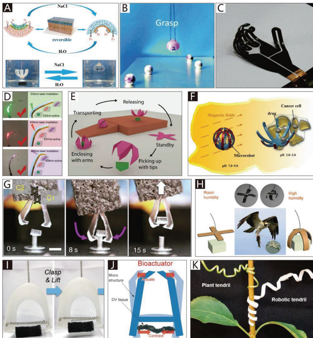
Figure 14. Soft grippers based on other smart materials. A) A salt-responsive bilayer hydrogel. Reproduced with permission. [296] Copyright 2017, American Chemical Society. B) A mimosa inspired bilayer hydrogel gripper. Reproduced with permission. [299] Copyright 2018, Royal Society of Chemistry. C) A polymer electrothermal hand. Reproduced with permission. [68] Copyright 2015, American Chemical Society. D) A light-sensitive soft finger. Reproduced with permission. [289] Copyright 2018, John Wiley and Sons. E) A programmable micrometer-scale robot. Reproduced with permission. [292] Copyright 2019, The American Association for the Advancement of Science. F) A pH-responsive hydrogel-based soft micro-robot. Reproduced with permission. [69] Copyright 2016, IOP Publishing. G) A small-scale soft gripper. Reproduced with permission. [293] Copyright 2013, Springer Nature. H) A soft gripper responded to humidity. Reproduced with permission. [294] Copyright 2019, Springer Nature. I) An electrothermal soft gripper. Reproduced with permission. [290] Copyright 2018, American Chemical Society. J) An insect muscle powered bio-actuator. Reproduced with permission. [300] Copyright 2016, Mary Ann Liebert, Inc. K) A soft tendril-inspired twining-type gripper. Reproduced with permission. [177] Copyright 2018, American Chemical Society.
