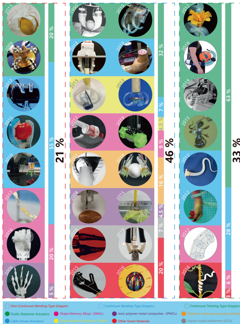
Figure 2. Non-continuum bending-type grippers (NBGs): A soft gripper with “pouch motors.” Reproduced with permission. [46] Copyright 2015, Mary Ann Liebert, Inc. A soft micro-gripper with four fingers. Reproduced with permission. [47] Copyright 2009, IEEE. A cable-driven manipulation with elastic finger joints. Reproduced with permission. [48] Copyright 2017, SAGE Publications. A gripper is driven by a single cable tendon. Reproduced with permission. [49] Copyright 2015, Mary Ann Liebert, Inc. An omni-purpose soft gripper incorporated with soft fingers and a suction cup. Reproduced with permission. [50] Copyright 2019, IEEE. A wireless folding gripper. Reproduced with permission. [51] Copyright 2017, The American Association for the Advancement of Science. A soft hand with a good bending capacity. Reproduced with permission. [52] Copyright 2016, Elsevier. A bionic finger is driven by IPMC actuators. Reproduced with permission. [53] Copyright 2006, IOP Publishing. Continuum bending-type grippers (CBGs): A flexible pressure-driven gripper. Reproduced with permission. [54] Copyright 1990, Cambridge University Press. A soft gripper is used to grasp aquatic mollusk. Reproduced with permission. [55] Copyright 2019, The American Association for the Advancement of Science. A precharged pneumatic soft gripper. Reproduced with permission. [56] Copyright 2018, Mary Ann Liebert, Inc. A soft wearable robot for hands. Reproduced with permission. [57] Copyright 2019, Mary Ann Liebert, Inc. A gripper is driven by SMPs. Reproduced with permission. [58] Copyright 2015, Springer Nature. Bidirectional SMPs. Reproduced with permission. [59] Copyright 2013, John Wiley and Sons. An SMA-based soft gripper. Reproduced with permission. [60] Copyright 2017, Elsevier. A gripper with SMA springs. Reproduced with permission. [61] Copyright 2019, IOP Publishing. A soft gripper based on DEMA. Reproduced with permission. [62] Copyright 2007, AIP Publishing. Hydraulically amplified self-healing electrostatic gripper. Reproduced with permission. [63] Copyright 2018, The American Association for the Advancement of Science. A microgripper is driven by IPMC. Reproduced with permission. [101] Copyright 2008, Springer Nature. A Venus flytrap-inspired microrobot consists of two IPMC actuators. Reproduced with permission. [65] Copyright 2015, Springer Nature. A micrometer-scale, light-driven plier. Reproduced with permission. [66] Copyright 2020, John Wiley and Sons. Electrically controlled soft gripper with three LCE
