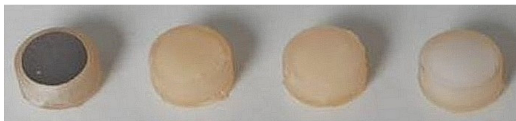
Figure 6. Investigated biomaterials: titanium, glass ionomer, composite, and Zn-containing polymer.
