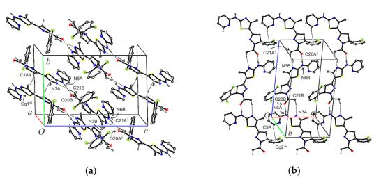
**Figure 8.** Two views of the unit cell (**a**) and (**b**) showing N—H···O and C—H···N hydrogen bonding and C—H···*Cg* intermolecular interactions in the crystal structure of **6**. The H atoms not involved in hydrogen bonds have been omitted for clarity; Cg1 = thiazole system, Cg2 = phenyl system.
