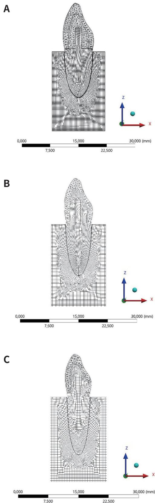
**Fig. 2.** Finite element mesh from (A) fat model, (B) medium model and (C) slim model.
