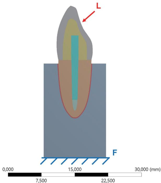
**Fig. 3.** Boundary conditions showing the loading region (L) and the fixation support (F).
