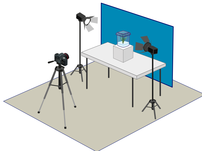
Figure 4. Schematic diagram of imaging station used to collect images of tissue culture vessels for this experiment.
