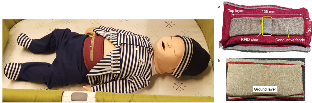
Figure 1. (left) A smart-fabric Bellyband and (right) Bellypatch can be integrated into wearable garments to enable wireless and passive biomedical monitoring in infants. (a) top and (b) bottom view of the Bellypatch.
