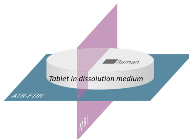
Fig. 1 Scheme of image positions relative to the tablet, provided by each imaging method used in this work.
