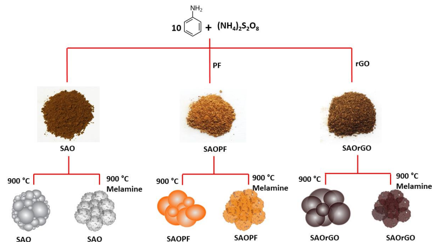
Scheme 1. A schematic representation of the preparation of macroporous carbon materials (MCMs).
