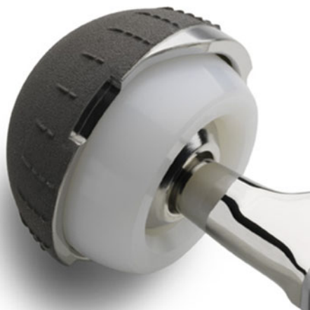
Fig. 1. DM cup: The mobile polyethylene insert is not constrained in the metal back constituting the large articulation. It is clipped over the femoral head (22- or 28-mm diameter) constituting the small articulation. Note the smooth aspect of the head–neck junction as well as the absence of an extraction hole
