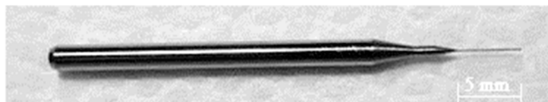
Figure 4. Commercially available spindle micro-tool without the screw slot. Diameter of shank: 3 mm. Diameter of tool: 0.15 mm.
