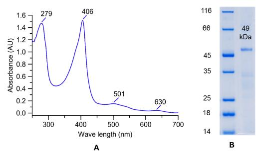
**Figure 3.** (**A**) UV–Vis absorption spectrum of purified XgrDyP in its resting state with the Soret band at 406 nm and additional bands at 279, 501, and 630 nm representing the  $\delta$ -,  $\beta$ -, and  $\alpha$ -bands, respectively. (**B**) SDS-PAGE of the purified X. grammica DyP (XgrDyP; right), left: protein marker.
