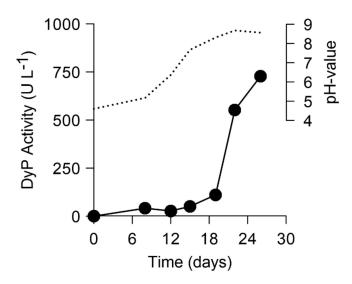
**Figure 1.** Time course of DyP production (black circles) by X. *grammica* in SPM medium; activity was measured with ABTS and  $H_2O_2$ , dotted lines—pH value.
