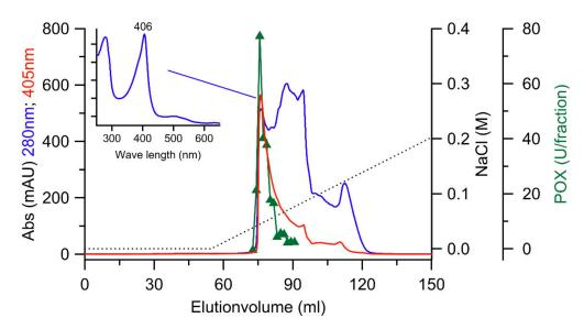
**Figure 2.** FPLC elution profiles of the last re-chromatographic purification step of XgrDyP using a MonoQ column (10 × 100 mm). Absorption (mAU) at 280 nm (blue $\rightarrow$ total protein) and 405 nm (red $\rightarrow$ heme), DyP activity (green), NaCl gradient (dashed line).
