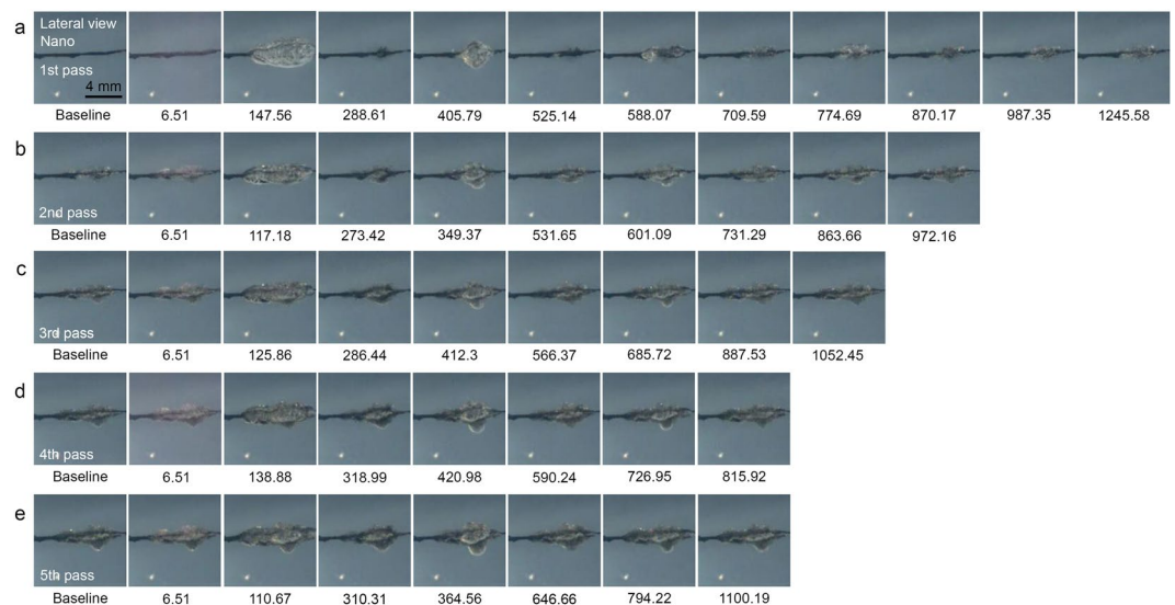
Figure 5. High-speed cinematography of nanosecond-domain Nd:YAG laser treatments on tattoo-embedded TM phantom. Captured frames present the development of PIZs after repeated courses of acoustic wave reflection and propagation immediately after nanosecond-domain Nd:YAG laser treatment at the laser fluence of 1.5 \text{ J/cm}^2 and a spot size of 7 mm over five pulses at 5 Hz. Lateral view; times are presented as \mu\text{sec} ; Nano, nanosecond-domain laser.
