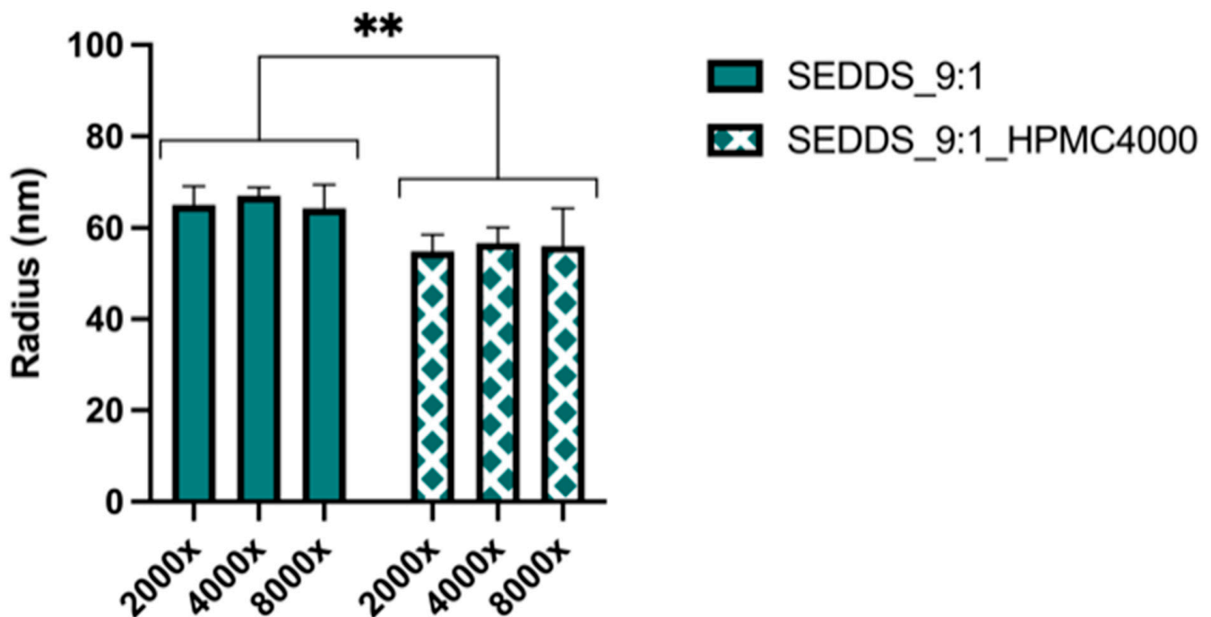
Figure 7. Droplet size SEDDS_9:1 and SEDDS_9:1_HPMC4000 after immersion in GISS phase III at different dilution factors i.e., 2000×, 4000×, and 8000× (mean ± SD, n = 3 ; ** p < 0.01 ).
