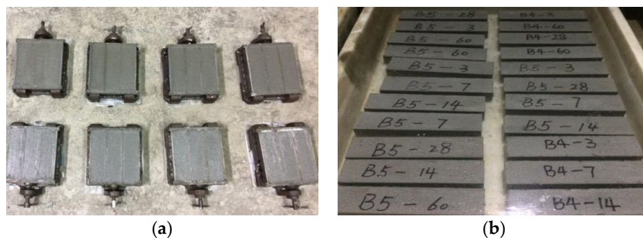
Figure 1. Sample preparation. (a) the test blocks in forming; (b) the test blocks in curing.
