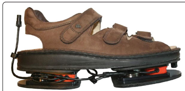
Figure 1 Instrumented shoes. Instrumented Shoes (right shoe). Each Force Shoe (left and right) has 2 sensors modules: one under the forefoot and one under the heel. A sensor module includes a Force/Torque Sensor and a Motion Tracker.
