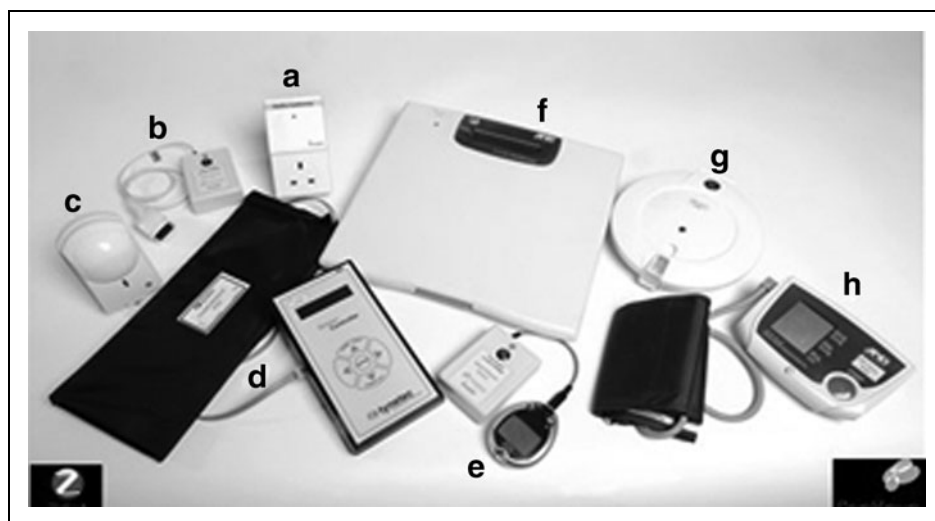
Fig. 2. Gateway and sensors used: (a) the gateway, (b) pulse oximeter, (c) PIR motion sensor, (d) bed sensor, (e) glucose meter, (f) weight scale, (g) medication dispenser, (h) BP meter. BP, blood pressure; PIR, passive infrared.
