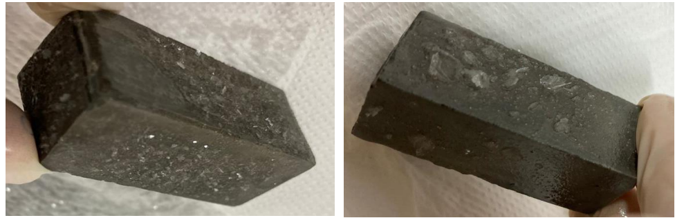
Figure 12. Photographs of products formed on TS surfaces after deposition for 120 days at 40 °C in 1 mol/L solutions, on the left TS deposited in nitrate solution, on the right in hydroxide.
