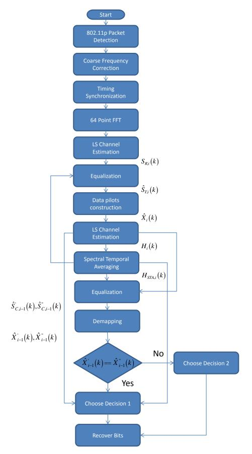
Figure 5. Process flow of the proposed algorithm.
