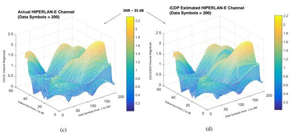
**Figure 10.** Actual and Estimated HIPERLAN-E channels: (a) Actual channel at SNR = 15 dB. (b) Estimated channel at SNR = 15 dB. (c) Actual channel at SNR = 35 dB. (d) Estimated channel at Signal-to-Noise Ratio (SNR) = 35 dB.
