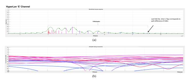
**Figure 11.** Multipath components of the HIPERLAN-E channel: (**a**) Bandlimited impulse response. (**b**) Multipath fading components after 850 µs.
