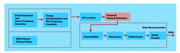
Figure 3. IEEE 802.11p receiver block diagram.
