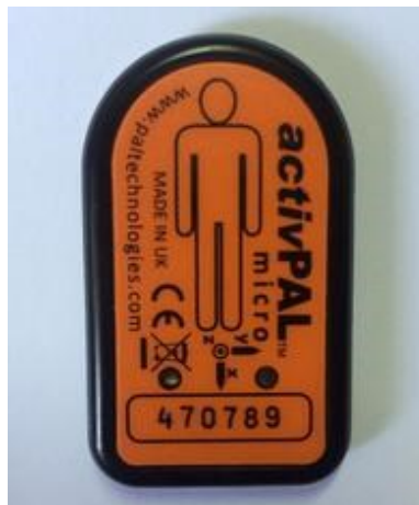
Figure 1. The activPAL™ micro accelerometer, with the figure on the front indicating the direction of attachment.
