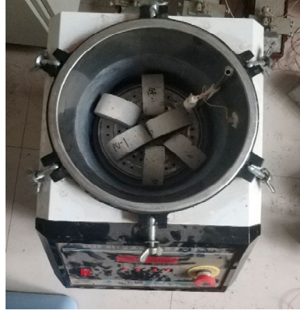
Figure 7. Instrument of vacuum water saturation.
