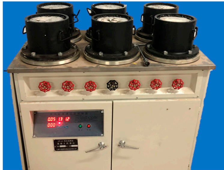
Figure 6. Instrument of permeability resistance of concrete.
