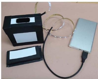
**Fig. (1).** Dark box made of matte cardboard is used to detect fluorescent signals using smartphone camera (*A higher resolution / colour version of this figure is available in the electronic copy of the article*).
