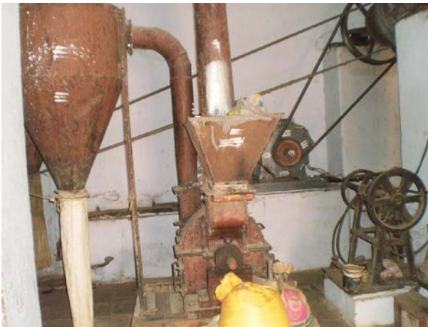
Fig. 7.6 Simple apparatus for expression of neem kernels.
