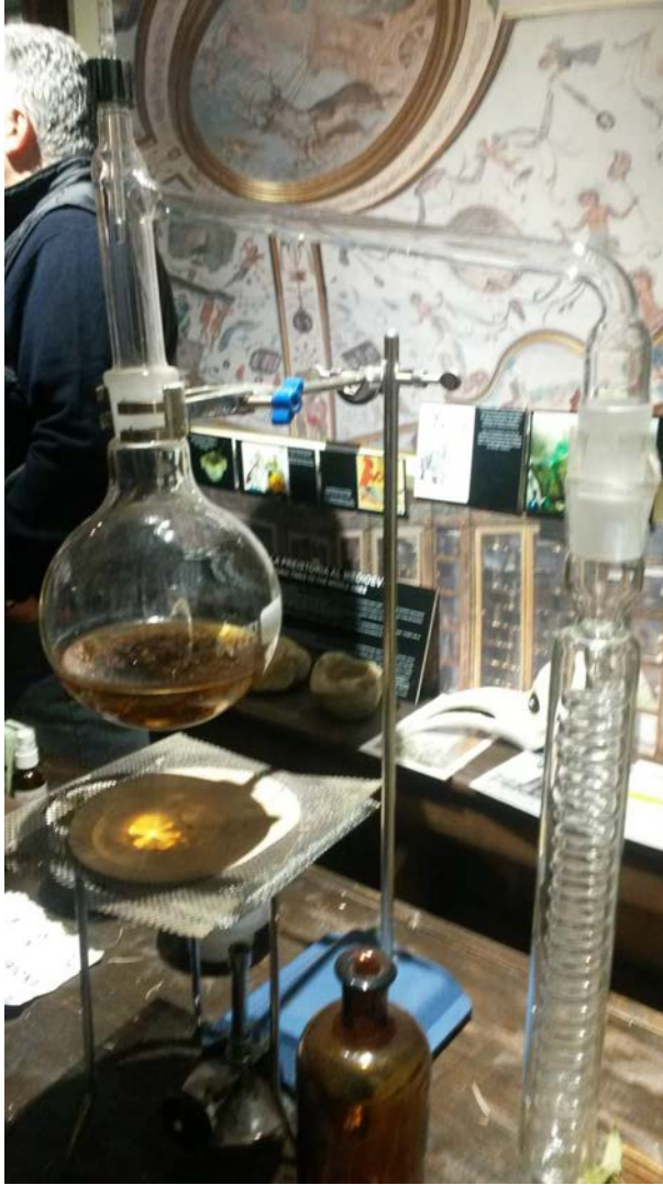
Fig. 7.1 A typical current apparatus for the production of essential oils by steam distillation.
