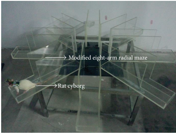
FIGURE 8: A side view of the modified eight-arm radial maze for automatic training. Two high plexiglass walls (40 cm \times 15 cm) have been added to each arm (60 cm \times 15 cm) to prevent the rat cyborg from climbing up the arm, and the width of each arm is set small enough to prevent the rat cyborg from turning around. Because the plexiglass walls is shorter than each arm, the rat cyborg can turn around at the tail end.
