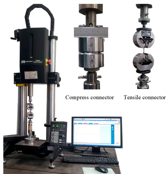
Figure 3. Schematic diagram of testing machine and compress/tensile connector.
