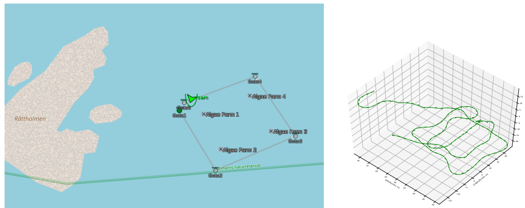
Figure 13. A mission plan to inspect the outside of the seaweed farm in Neptus (left). In Stonefish, the AUV follows 4 waypoints in straight lines around the extremities of the farm (shown as crosses in the Neptus figure) at a depth of 2.5 m, and then inspects the inside (right). Since this farm has two parallel algae lines, the vehicle does three close-by passes after the initial survey. The vehicle then moves out of the farm.
