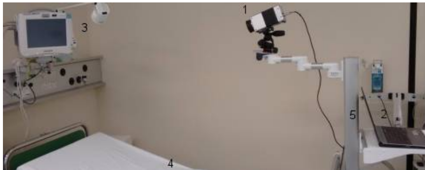
Figure 1. The experimental setup in the post-anesthesia care unit (PACU). (1) Long-wave infrared camera, VarioCAM ® HD head 820 S/30 mm (Infratec GmbH, Dresden, Germany). (2) Laptop. (3) Philips IntelliVue MP30 monitor (Philips Electronics N.V., Amsterdam, the Netherlands). (4) Patient bed. (5) Rolling rack.
