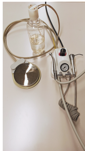
Figure 2. Presentation of the air turbine and control apparatus used in the present study. The pressurized water tank used to generate the air-water cooling spray for the turbine handpiece is seen on the upper part. The handpiece cord was afterwards inserted inside the chamber and sealed, for the turbine to operate inside the patient phantom.
