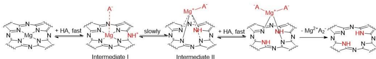
Figure 2. The acidoprotolytic mechanism of dissociation of Mg complexes in organic solvent in presence of acid HA. Based on ref. [29].
