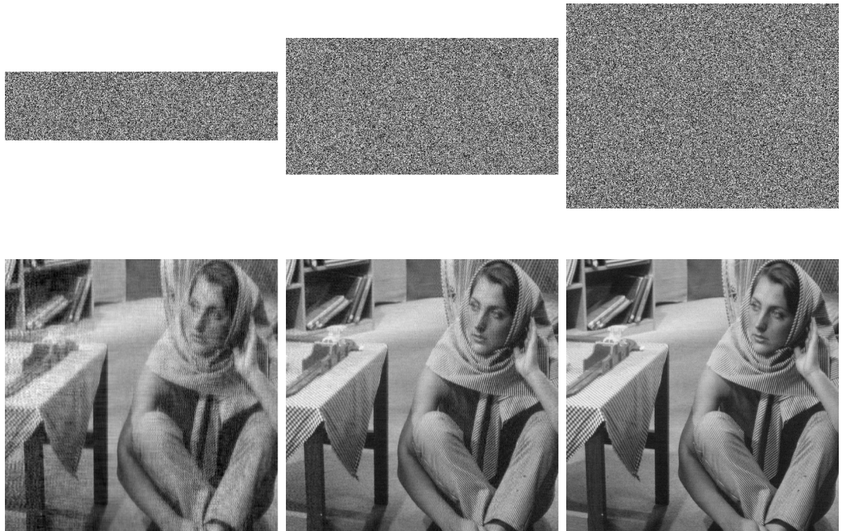
Fig 6. The encryption images of Barbara and their recovered images with different CRs of 0.25, 0.5 and 0.75. The first row shows their compressed and encrypted images by QSBLA while the second row shows their corresponding recovered images.
