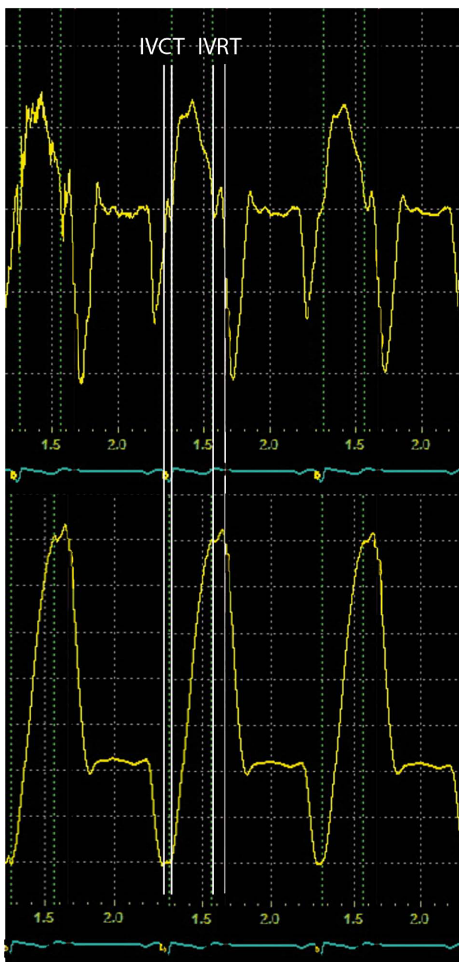
Figure 1 Typical LV longitudinal myocardial velocity curves (top) obtained with colour TD from the basal segment of septum (insertion). Integration of the velocity curves over time yielded the corresponding longitudinal myocardial displacement curves (bottom). Isovolumic contraction time (IVCT) and isovolumic relaxation time (IVRT) are indicated.
