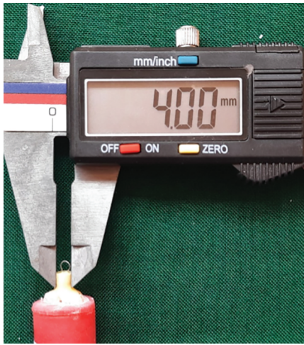
Fig. 1: Diameter of composite with loop for tensile loading
