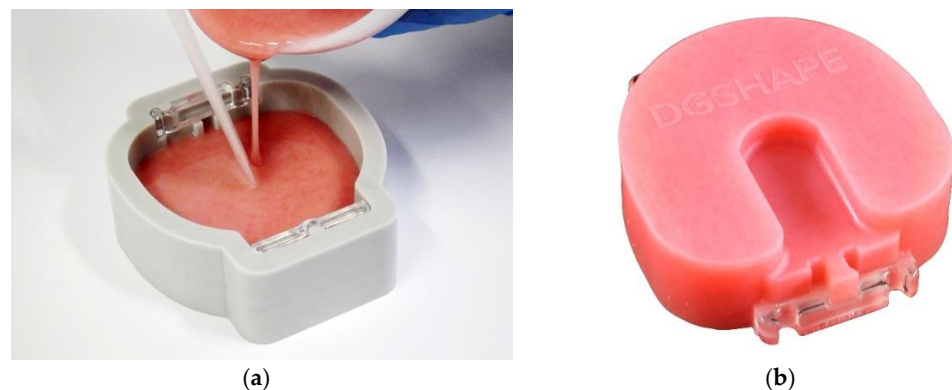
Figure 2. Manufacturing method of the block body. After mixing the self-polymerizing resin (Fit Resin; Shofu) at the standard powder ratio, we poured it into the dedicated tray of the denture cutting time reduction kit (CA-DK1; DGSHAPE): (a) pouring technique; (b) completed block body.
