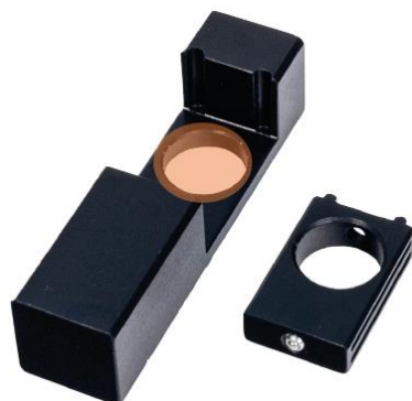
Figure 14. Image of the solid sample holder utilized for membrane analysis.
