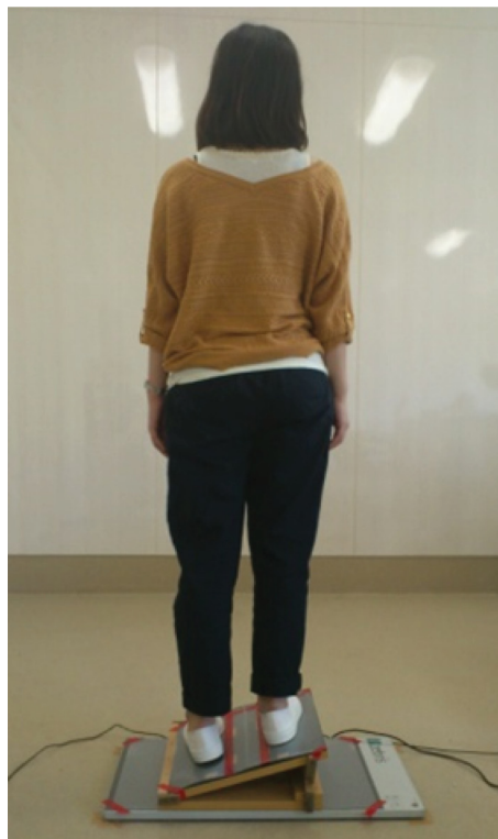
Fig. 1. Participant stood on a sideward slope, and the Zebris system was used to measure total length of the locus and body sway area.
