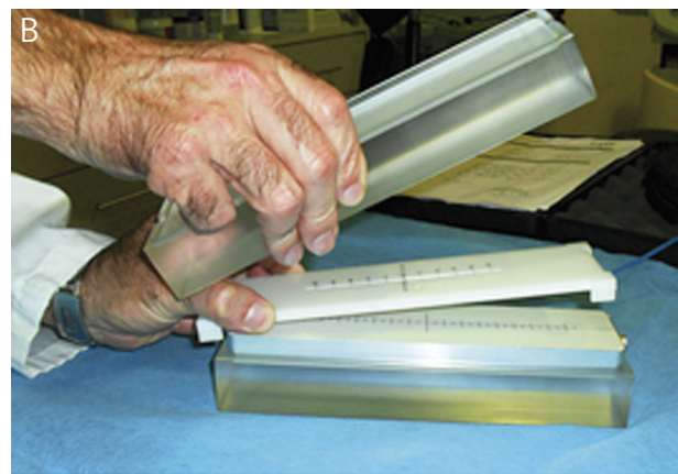
Fig. 1. A) Left-right: PMMA block, Nucletron insert to allocate the 10 selectSeed™, PTW SourceCheck (without the PTW insert), PMMA block (B) Mounting the set-up. Bottom-top: PMMA block + SourceCheck + Nucletron insert + PMMA block
