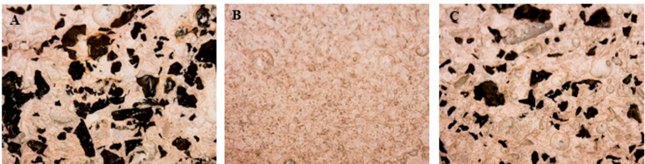
Figure 9. Sections of the (A) TR F sample (sample 1), (B) P sample (sample 10), (C) P/TR F sample (sample 11). The cross-section of these samples was analyzed by optical microscope after flexural rupture of the specimens.
