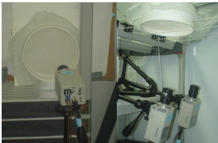
Fig. 3 Video cameras positioned in front of vertically oriented arena (left panel) and below horizontally oriented arenas (right panel)
