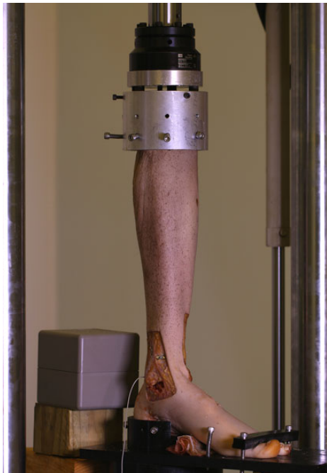
Figure 2. Overall test setup showing motion-tracking source, tibial sensor, and test fixture. The upper fixture applied torsion and compression to the proximal tibia, while the lower fixture held the foot stationary.
