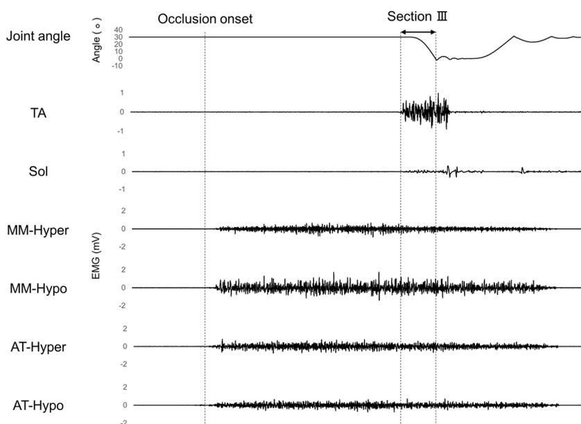
**FIGURE 2** Raw data tracing EMG of each muscle. Raw data in the Max condition of the joint movement task from one representative subject. The top graph shows the joint motion from 30° of ankle joint plantar flexion to 0° of plantar dorsiflexion. The graphs below show the EMG of each muscle. AT, anterior temporalis muscle; EMG, electromyography; MM, masseter muscle; Sol, soleus muscle; TA, tibialis anterior muscle.
