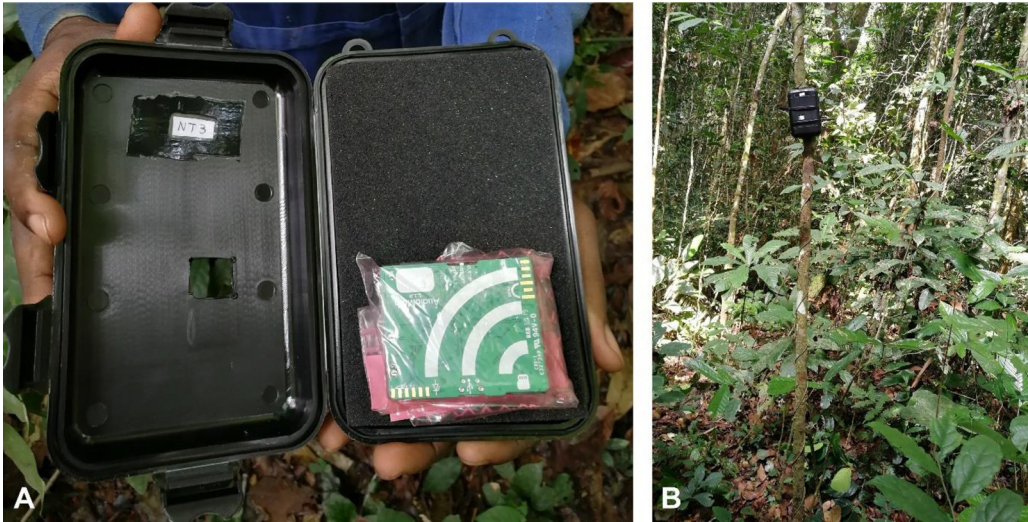
Fig. 2. Audio sampling design. A) An AudioMoth bioacoustics sensor wrapped in a zip lock bag, placed in a protective, labelled case with foam in the back to keep the sensor in place and a small hole in the front at the location of the microphone. B) A sensor deployed in the forest, attached to a tree at a height of 2 m, orientated at 90°.
