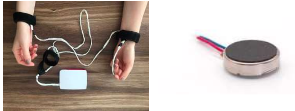
Figure 4. Raspberry Pi 4 with tactile module integrated and the vibration motor 1027 [22].
