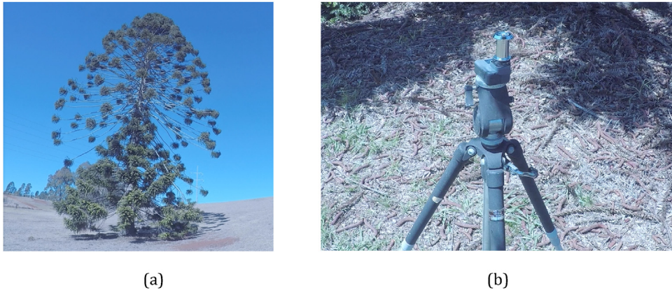
Fig. 1. (a) A growing tree canopy that continually refreshes its leaf cover and grows in size can provide sustained solar ultraviolet protection for the life of the tree. Araucaria bidwillii , 19.0 m high and canopy diameter 14.1 m, is shown at its measurement location, 27.6014°S, 151.9408°E. (b) Experimental apparatus including tripod, video camera, neutral density filter and fish eye lens attachment are used to measure the effective sky view underneath Araucaria bidwillii .
