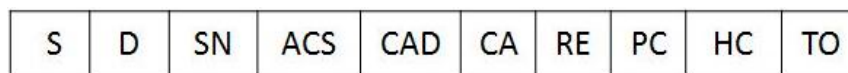
Figure 2. RREQ packet structure. S: Source; D: Destination; SN: Sequence Number; ACS: Available Channel Set; CAD: Channel Access Duration; CA: Channel Assigned; RE: Residual Energy; PC: Path Cost; HC: Hop Count; TO: Timeout.
