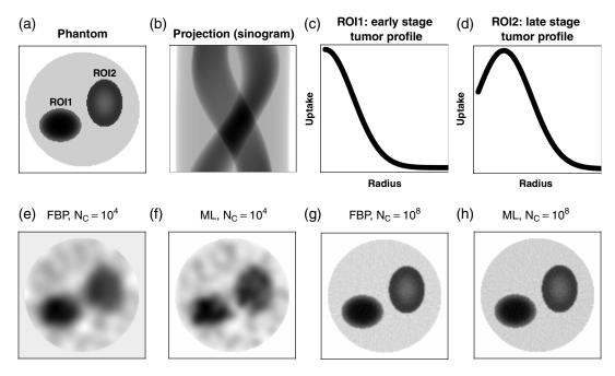
**Fig. 8** (a)–(d) 2-D phantom data and (e)–(h) reconstruction examples, using filtered backprojection (FBP) and maximum likelihood (ML) at low ( $N_C = 10^4$ ) and high ( $N_C = 10^8$ ) count levels. Note that reconstructions are set to zero in background (defined as the region with no attenuation).
