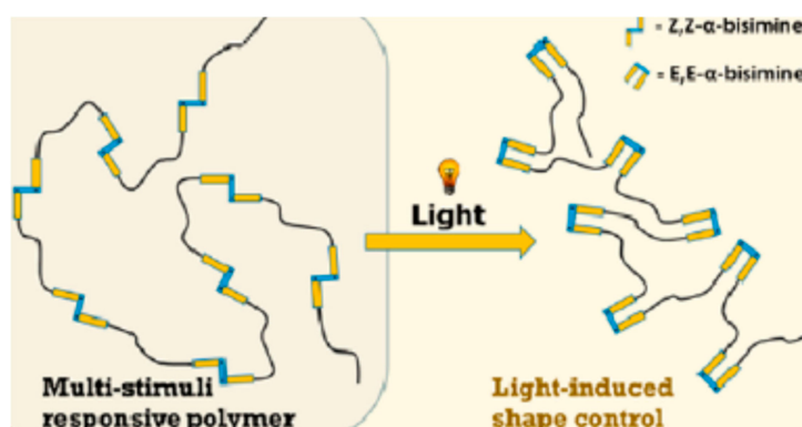
Figure 9. Schematic illustration of the controlled switching of size/shape with light via photoisomerization of an ADMET-polymer containing main-chain N-alkyl \alpha -bisimine units. Reprinted from [39] with permission.
